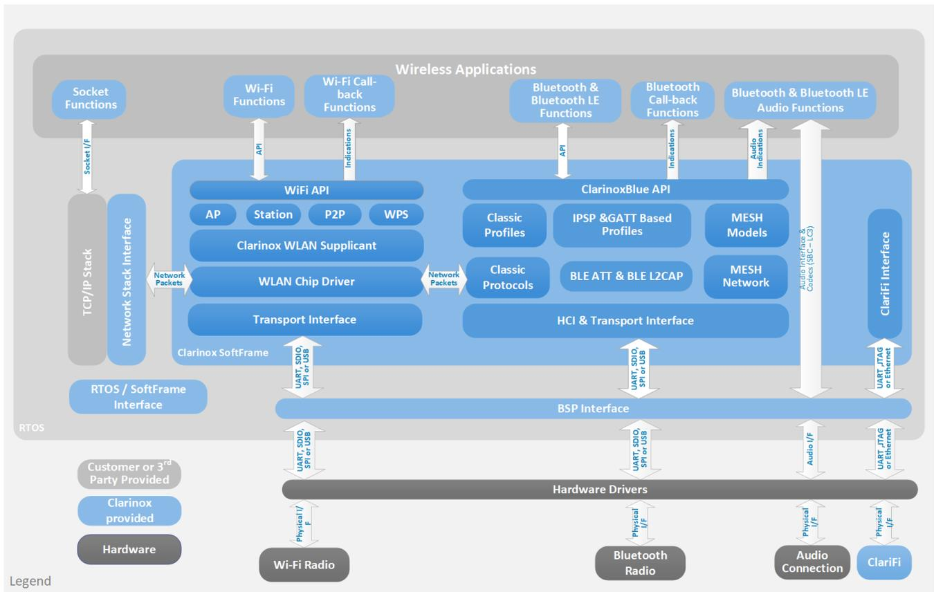
Fig. 2. Architecture of connectivity solution within abstraction based architecture
